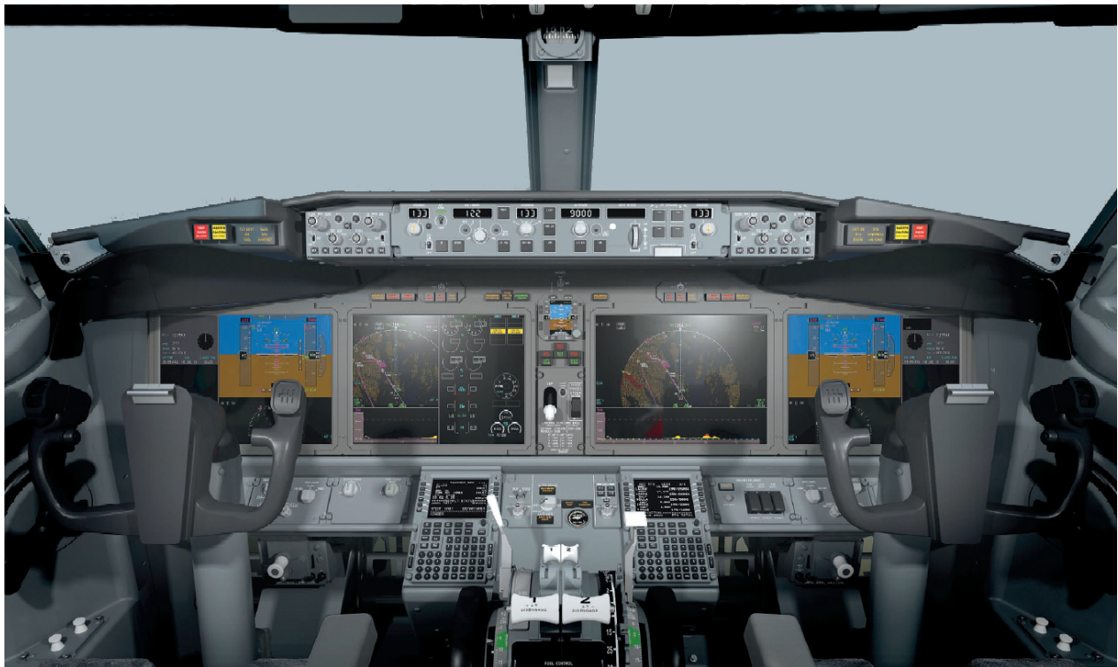
737 MAX Flight Deck, including pilot and co-pilot's control yokes and columns (Boeing).
