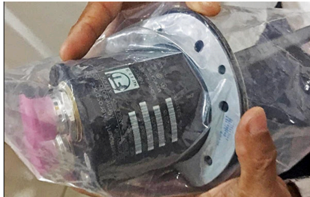
Angle of attack sensor from Lion Air crash. (TimothyMcLaughlin/Washington Post)
