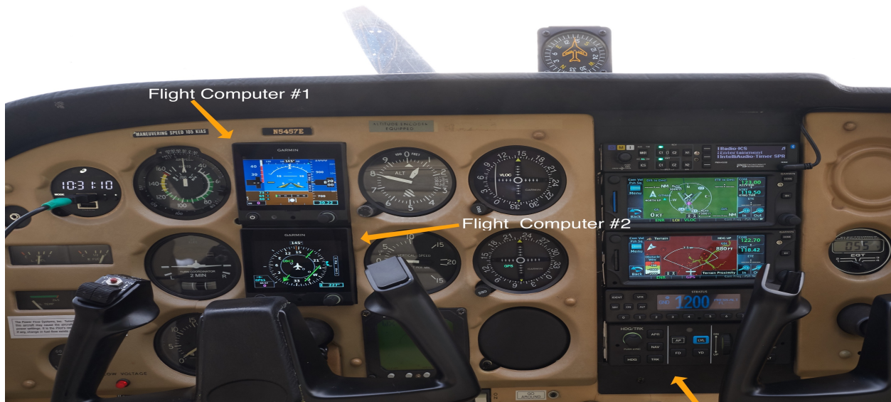
My Cessna 172's control panel. Note location of autopilot circuit breaker. Also note autopilot disconnect switch (red button atop left-hand side of pilot's yoke). Control cables physically link the control yokes to the flying surfaces in my plane.
