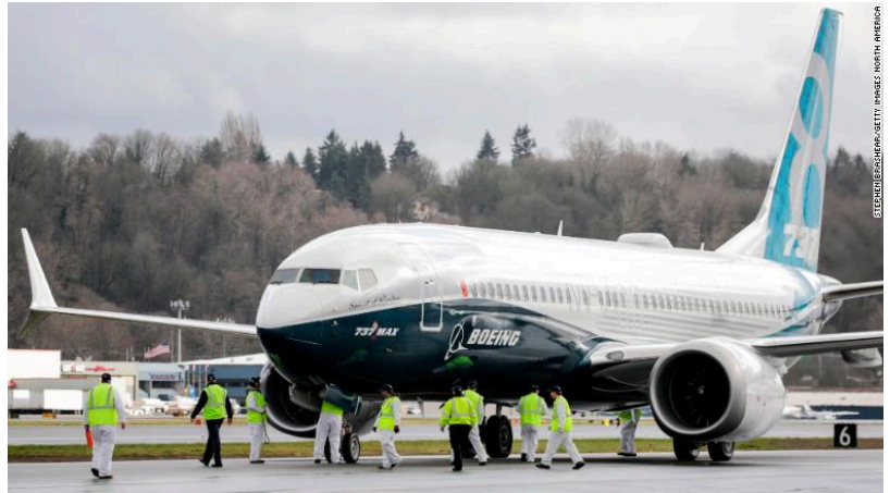
737 MAX with CFM LEAP engines. Note "ovalization" of intake AND placement of engine ahead and slightly above wing. This placement is what causes the "pitch up" when power is applied (Boeing).
